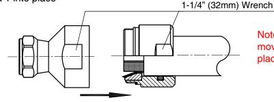
Note: Be sure Back Nut does not move when screwing Body into place.
