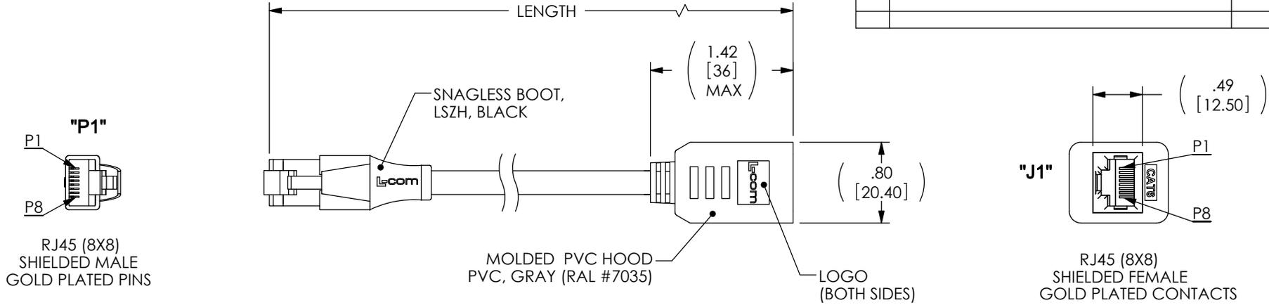
(4) SHIELDED TWISTED PAIRS, CAT6 MODULAR CABLE, CONDUCTORS: 26AWG STRANDED COPPER, OVERALL SHIELD: ALUMINUM MYLAR, OUTER JACKET: PVC, GRAY (RAL #7035)
