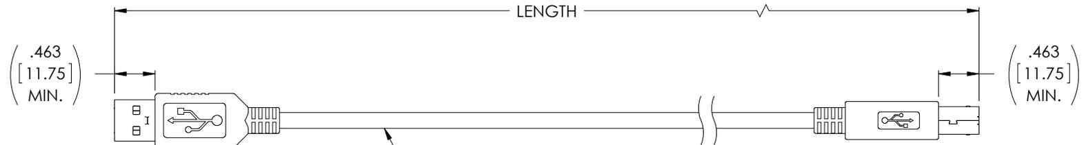
ONE 28AWG STRANDED TINNED COPPER TWISTED PAIR
